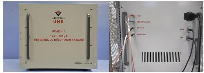
Fig. 12. The ULCS device front and back view.
