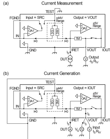
Fig. 2. Configurations for extending the current range of the 3 G $\Omega$  ULCA up to  $\pm 5$   $\mu$ A. (a) Current measurement with a current source as device under test (DUT), (b) current generation with an amperemeter as DUT. In (b) a star-shaped wiring for voltage source  $V_S$  and voltmeter is recommended to minimize parasitic series resistance.
