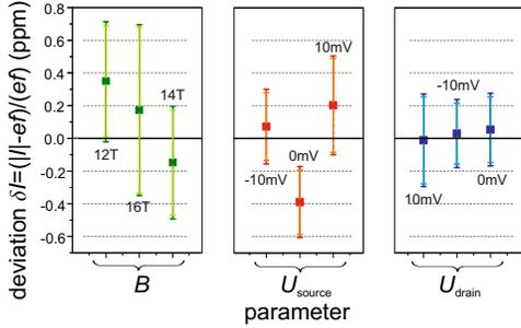
Fig. 3. Resulting deviation  $\delta I$  from  $ef$  derived from averaging a particularly chosen number of precision points such as shown in Fig. 2(b) for parameter variation of magnetic flux density  $B$ , bias voltage of source  $U_{\text{source}}$  and drain  $U_{\text{drain}}$ . Light Error bars reflect Type A uncertainty, dark Error bars combined uncertainties (all for  $k = 1$ ).
