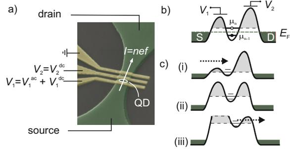
Fig. 1. (a) False-color SEM micrograph of a single-electron pump with descriptions. (b) Sketch of the dynamic QD which is electrostatically defined via top-gates. Fermi level and energy levels of the QD are indicated. (c) Process of electron transfer sketched in three phases, (i) loading electrons from the source lead, (ii) isolation of the quantum dot, and (iii) ejecting electrons to drain.
