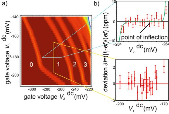
Fig. 2. (a) Contour-line plot of the deviation of current. Regions of 0, 1, 2, and 3 transferred electrons are labeled. (b) Precision measurements realized in regions marked in (a), diagrammed in deviation from  $ef$ . Error bars reflect Type A uncertainty ( $k = 1$ ). Green graph shows a fit proposed in [10].
