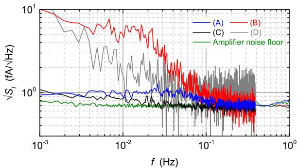
Figure 2. Current noise levels of four different 2 m long cables measured with the low-noise current amplifier prototype ( $0.7 fA/\sqrt{Hz}$  white noise). The noise level of (B) and (D) strongly increases at frequencies below about 0.1 Hz, while (A) and (C) show only small degradation. The best cable (C) has PE as dielectric.
