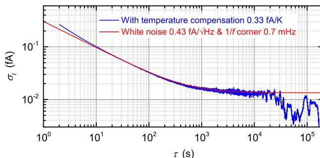
Figure 1. Allan deviation plot of the amplifier signal. Effects caused by temperature fluctuations are compensated by taking into account the amplifier's temperature coefficient of  $0.33 \text{ fA}/\text{K}$ . The red fit curve is calculated from the measured noise spectrum. For the measurement, a total transresistance  $A_{\text{TR}}$  of  $1 \text{ T}\Omega$  was chosen.
