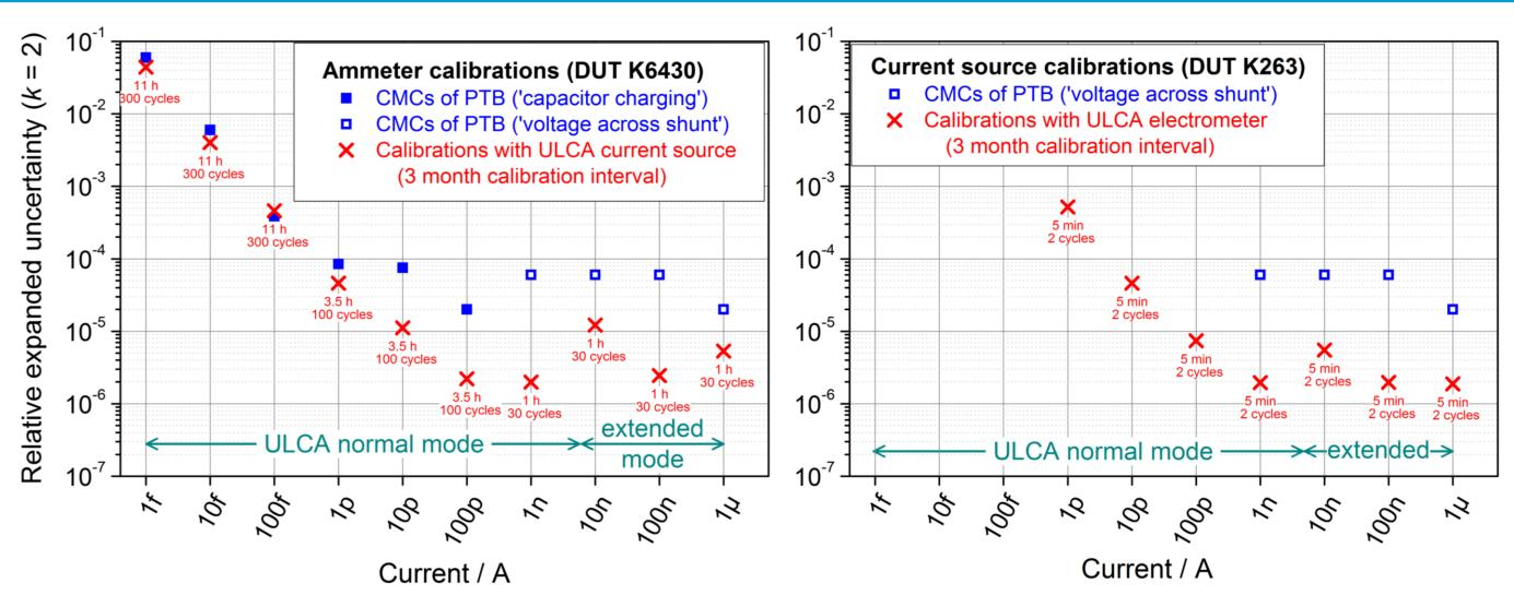
In summary, the ULCA provides several significant advantages compared with other calibration methods for electrometers and low-current sources:
